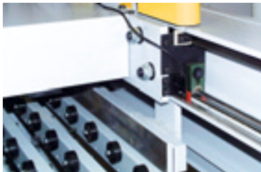
The measuring system consisting of magnetic sensor / band is a modern and economic alternative to standard rotary encoder systems with rack and pinion.
